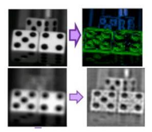
The angle-sensitive image sensor can provide range mapping for use in 3-D applications, and also allows images to be refocused after they are taken.
