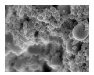
Hydroxyapatite nanoparticles are incorporated into multilayer coatings for faster bone tissue growth. Image courtesy of the Hammond Lab
