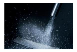
Shot is fi red from a blasting gun at a ceramic leaf spring to correct its shape or cause specifi c warping as desired. Credit: Fraunhofer IWM, Felicitas Gemetz
