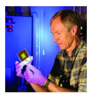
Los Alamos scientist Meiring Nortier holds a thorium foil test target for the proof-of-concept production experiments. Research indicates that it will be possible to match current annual, worldwide production of Ac-225 in just two to five days of operations using the accelerator at Los Alamos and analogous facilities at Brookhaven.
