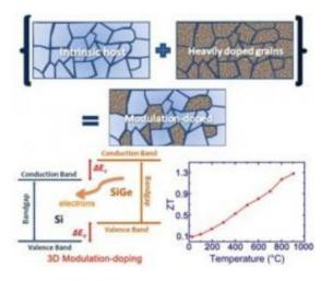
While long valued for high-temperature applications, the bulk alloy semiconductor SiGe hasn't lent itself to broader adoption because of its low thermoelectric performance and the high cost of Germanium. A novel nanotechnology design created by researchers from Boston College and MIT has shown a 30 to 40 percent increase in thermoelectric performance and reduced the amount of costly Germanium. Credit: Nano Letters
