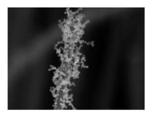
Decoration with nanoparticles creates intricate surface patterns full of nooks and crannies, twists and turns that greatly improve surface area. Credit: Stanford Nanocharacterization Laboratory
