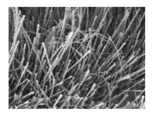
Prof. Xiaolin Zheng at Stanford has discovered a new way to "decorate" nanowires with coatings of metal nanoparticles that greatly improve surface area. The decorated nanowires look like tiny pipe cleaners. Credit: Stanford Nanocharacterization Laboratory
