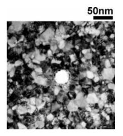
This transmission electron micrograph shows a solid-state nanopore: The white circle in the middle of the picture. The otherwise patchy-looking structure results from the polycrystalline nature of a gold film that was evaporated onto the silicon nitride membrane (which cannot be seen). Credit: Rant group, TU Muenchen Copyright TU Muenchen
