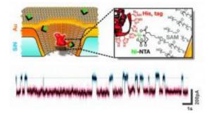
This schematic illustration shows a gold-coated solid-state nanopore that is chemically modified with a single receptor capable of binding protein molecules with a specific set of amino acid residues. An exemplary current-vs.-time trace shows the transient binding of single proteins. Credit: Rant group, TU Muenchen, Copyright TU Muenchen.
