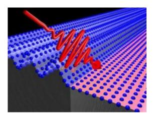
A femtosecond pulse of infrared laser light "pumps" the atomic lattice in vanadium dioxide, inducing a phase transition. Credit: Courtesy of Fritz Haber Institute
