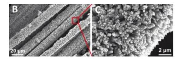
Scanning electron microscope images of TiO2 nanorod arrays uniformly covering the carbon fibers. Image credit: Guo, et al. ©2012 American Chemical Society
