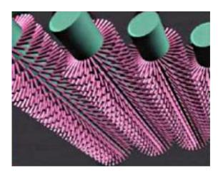
Illustration of TiO2 nanorod arrays on carbon fibers fabricated by the "dissolve and grow" method. Image credit: Guo, et al. ©2012 American Chemical Society
