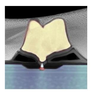
A cross-section of an experimental compound-semiconductor transistor developed by Jesus del Alamo's group at MIT's Microsystems Technology Laboratories. Image courtesy of Jesus del Alamo
