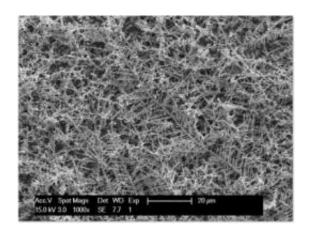
Fractal silver structures grown by electrochemical reduction of silver nitrate on a fluorine doped tin oxide film. These structures could be the basis of a new type of solar cell. Credit: Frank Osterloh, UC Davis
