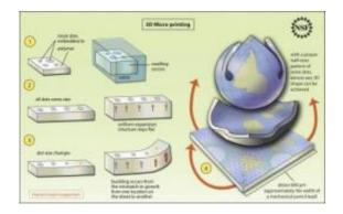
Controlling growth in a polymer system at the micro-scale with a technique akin to half-tone printing, the polymer swells like a sponge when exposed to water. Printing "resist dots" in the polymer substrate creates points that will not swell. When the dot size changes, buckling occurs from the mismatch in growth from one area to another. With a proper half-tone pattern of resist dots, almost any 3-D shape can be achieved. Credit: Zina Deretsky, National Science Foundation
