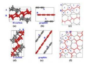
Crystal structure of H-carbon(a), initial AB stacking graphite supercell for Hcarbon (b) and side view containing five and seven carbon rings of H-carbon (c). Crystal structure of S-carbon (d), initial AB stacking graphite supercell for Scarbon (e) and side view containing five and seven carbon rings of S-carbon (f). Image from arXiv:1203.5509v1
