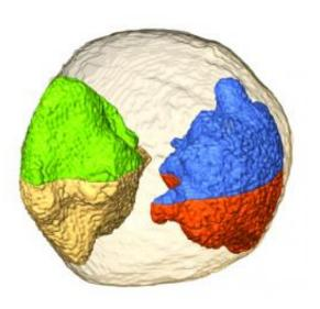
Jianwei Miao and colleagues have developed an electron tomography method to image the 3-D structure of a gold nanoparticle at a resolution of 2.4 angstroms. Individual atoms are observed in some regions of the particle and several grains are identified in three dimensions. In the figure, the four three-dimensional grains (green and gold; blue and red) form two pairs of twin boundaries inside the nanoparticle. Credit: Jianwei Miao/UCLA Physics & Astronomy, CNSI
