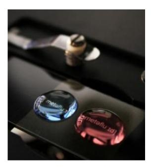
Although chemically alike solutions of right- and left-handed nano spiral staircases interact specifically with circular polarized light. The nano spiral staircases were built up using the DNA-origami method. Credit: TIM Liedl / LMU
