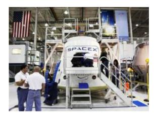
SpaceX and NASA conducted a daylong review of the Dragon crew vehicle layout using the Dragon engineering model equipped with seats and representations of crew systems. Credit: SpaceX
