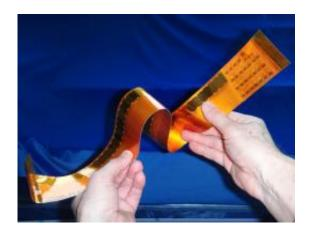
To map the pressure distribution on the wings as Europe's Hermes spaceplane returned through the atmosphere, a new sensor was developed for ESA based on super-thin piezoelectric materials. They have a special property that converts physical effects like vibration and pressure into minute electric pulses. Credits: Mirow Systemtechnik GmbH
