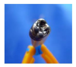
Piezoelectric materials painted on a tooth to measure the forces exerted by the brush on the molar. Credits: Mirow Systemtechnik GmbH
