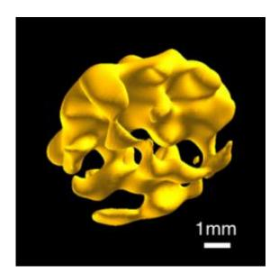
Yale University researchers have developed a new way of seeing inside solid objects. The technique, a novel kind of magnetic resonance imaging (MRI), creates three-dimensional images of hard and soft solids based on signals emitted by their phosphorus content. The image here shows the interior spongy bone of a rabbit femoral head, or the "ball" of the rabbit's hip bone.
