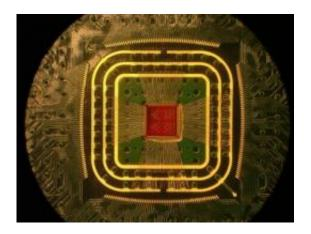
This is a photograph of the Columbia Engineering team's custom multichannel CMOS preamplifier chip, attached to a circuit board with thin gold wirebonds. Credit: Columbia Engineering
