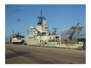
The Thomas G. Thompson and the Marcus G. Langseth at the Navy Pier in Guam. The Thompson laid seismic instruments, which are stacked and ready on its deck, and the Langseth then sailed transects over the instrumented area, firing its airgun array and recording the reflections from subsurface rock layers. Credit: DOUG WIENS
