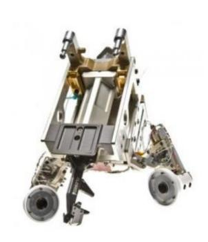
During the RRM Gas Fittings removal task, mission operators direct Dextre to use the Wire Cutter Tool to cut a wire. Credit: (NASA/SSCO)
