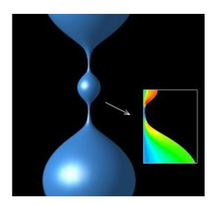
Simulations and high-speed visualization reveal a synergistic effect between chemical additives that can lead to the formation of satellite droplets during crop spraying. Emission of satellite droplets - shown here between two main drops - is also detrimental in a number of applications ranging from food processing to rocket propulsion systems. (Purdue University image)
