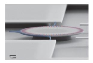
Image of an optical ring resonator, taken with a scanning electron microscope. CreditL: K. Srinivasan, NIST
