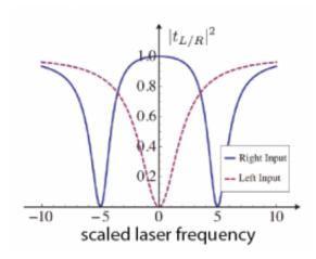
Theoretical calculation of light transmission (y-axis) through the waveguide when the optical resonator is operated as a diode. For a certain range of laser frequencies, the left moving light is attenuated, while light traveling from the right is transmitted. Credit: Figure courtesy of authors; a modified version
