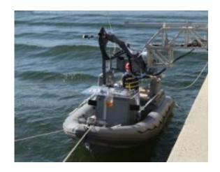
Positioned alongside a stationary platform, under simulated sea conditions, the USV Sea Fox receives fuel from a robotic fluids transfer arm via magnetic refueling fitting (shown here mounted in the forward bow section of the vessel). Credit: US Naval Research Laboratory
