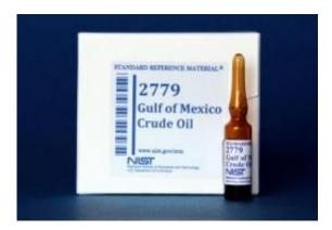
Gulf oil: Collected directly from the Macondo well during the Deepwater Horizon disaster and rigorously tested and measured by NIST and NOAA, NIST SRM 2779 will serve as a vital quality control for environmental impact analyses of the Gulf. Credit: L. Sander/NIST
