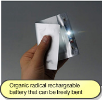
Organic radical rechargeable battery incorporated in cards
