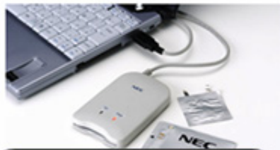
Organic radical rechargeable battery incorporated in cards
