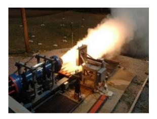
Mar. 14 test of a small solid rocket motor designed to mimic NASA's Space Launch System booster. Credit: NASA/MSFC
