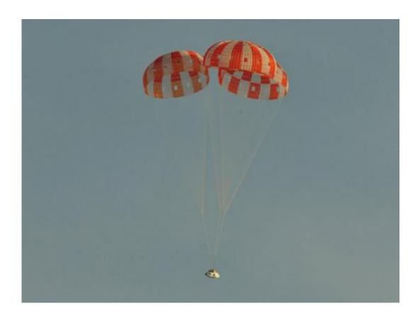
A test model of the Orion spacecraft with its parachutes was tested high above the skies over Arizona on Feb. 29. This particular drop test examined the wake - or the disturbance of the air flow behind Orion - that is caused by the spacecraft. This was the latest in a series of parachute drop tests conducted by NASA at the U.S. Army's Proving Grounds in Yuma, Ariz. Photo credit: NASA
