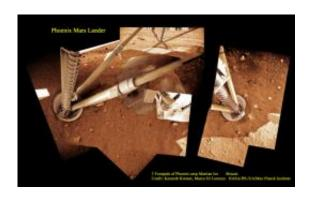
3 Footpads of Phoenix Mars Lander atop Martian Ice Phoenix thrusters blasted away Martian soil and exposed water ice. Proposed Mars InSight mission will build a new Phoenix-like lander from scratch to peer deep into the Red Planet and investigate the nature and size of the mysterious Martian core. Credit: Kenneth Kremer, Marco Di Lorenzo, Phoenix Mission, NASA/JPL/UA/Max Planck Institute
