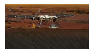
NASA's proposed Mars InSight (Interior exploration using Seismic Investigations, Geodesy and Heat Transport) Lander. InSight is based on the proven Phoenix Mars spacecraft and lander design with state-of-the-art avionics from the Mars Reconnaissance Orbiter (MRO) and Gravity Recovery and Interior Laboratory (GRAIL) missions in this artist rendition. Credit: JPL/NASA
