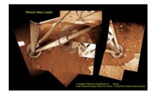
3 Footpads of Phoenix Mars Lander atop Martian Ice Phoenix thrusters blasted away Martian soil and exposed water ice. Proposed Mars InSight mission will build a new Phoenix-like lander from scratch to peer deep into the Red Planet and investigate the nature and size of the mysterious Martian core. Credit: Kenneth Kremer, Marco Di Lorenzo, Phoenix Mission, NASA/JPL/UA/Max Planck Institute
