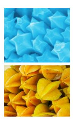
Gold nano particles, top, created by the Rice University lab of Eugene Zubarev take on the shape of starfruit, below, in a chemical bath with silver nitrate, ascorbic acid and gold chloride. Credit: Zubarev Lab/Rice University
