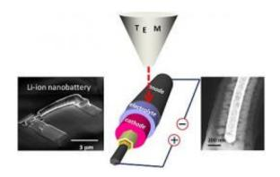
Using a transmission electron microscope, NIST reearchers were able to watch individual nanosized batteries with electrolytes of different thicknesses charge and discharge. The NIST team discovered that there is likely a lower limit to how thin an electrolyte layer can be made before it causes the battery to malfunction. Credit: Talin/NIST
