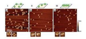
DNA origami: NIST researchers made three DNA origami templates designed so that quantum dots would arrange themselves: (a in the corners, b) diagonally (three dots), and (c in a line (four dots). The researchers found that putting the quantum dots closer together caused them to interfere with one another, leading to higher error rates and lower bonding strength. Credit: Ko/NIST
