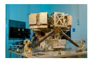
This is the flight Mid-Inrared Instrument (MIRI) at the Rutherford Appleton Laboratory in England. Credit: RAL
