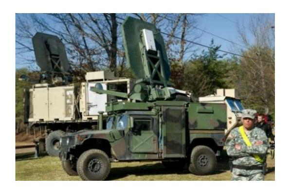
Two styles of US Marine Corps trucks are seen carrying the Active Denial System, March 9th, 2012, at the US Marine Corps Base Quantico, Virginia. The non-lethal weapon projects a strong electromagnetic beam up to 1000-meters. The beam creates heat so uncomfortable the natural response is to flee
