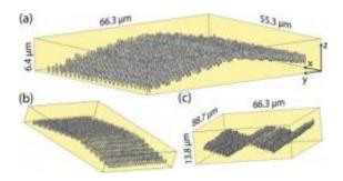
A new laser fabrication technique developed at Harvard allows for the creation of precisely arranged silver nanoparticles that are disconnected in 3-D and supported by a polymer matrix. The new technique may prove critical in the development of metamaterials. Credit: Image courtesy of Kevin Vora
