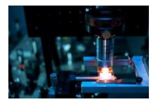
The experimental setup in professor Eric Mazur's laser laboratory at Harvard. Using femtosecond lasers, Mazur and colleagues have developed a new nanofabrication process for use in creating metamaterials. Credit: Eliza Grinnell, Harvard SEAS
