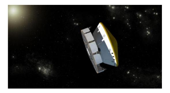
This is an artist's concept of NASA's Mars Science Laboratory spacecraft during its cruise phase between launch and final approach to Mars. The spacecraft includes a disc-shaped cruise stage (on the left) attached to the aeroshell. The spacecraft's rover (Curiosity) and descent stage are tucked inside the aeroshell. Credit: NASA/JPL-Caltech
