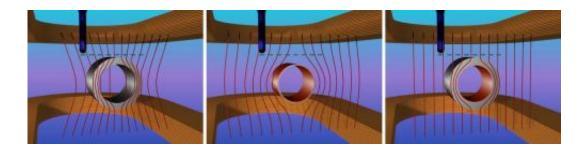
The ferromagnet attracts magnetic field lines (left), the superconductor repels magnetic field lines (middle), and the superconductor-ferromagnetic bilayer cloaks a magnetic field (right). An object inside the cloak would be magnetically undetectable. Image courtesy of J. Prat-Camps, C. Navau, A. Sanchez
