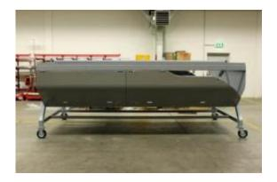
Although this diesel engine housing for trains is made of a light polyurethanebased material, it is nonetheless capable of withstanding extreme stresses. Credit: Fraunhofer ICT
