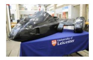
This is the fairing (the bodywork that covers the chassis and engine) that the team are working on. Credit: University of Leicester
