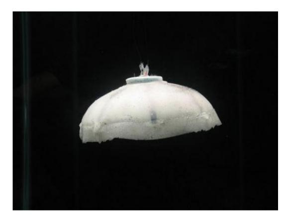
This undated photo released by the BMDL and CEHMS labs at Virginia Tech in Blacksburg, Virginia, show the robotic jellyfish "Robojelly." Scientists are developing a robotic jellyfish which uses the limitless energy of sea water to power its movement, according to US Navy-backed research.
