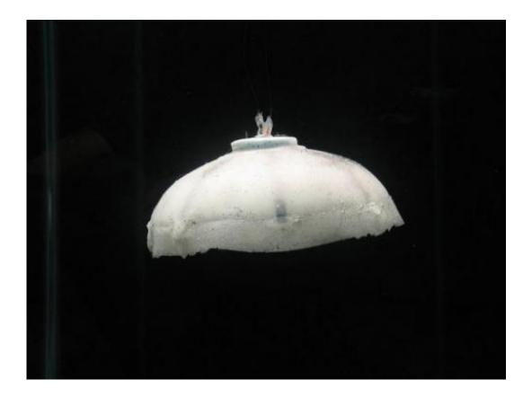
This undated photo released by the BMDL and CEHMS labs at Virginia Tech in Blacksburg, Virginia, show the robotic jellyfish "Robojelly." Scientists are developing a robotic jellyfish which uses the limitless energy of sea water to power its movement, according to US Navy-backed research.
