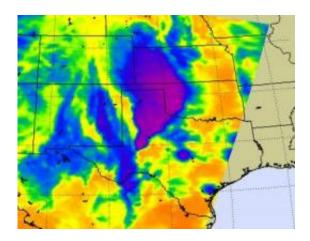
The AIRS instrument onboard NASA's Aqua satellite captured an infrared image that showed cloud top temperatures in the severe frontal system over Texas and western Oklahoma on March 19 at 0853 UTC (4:53 a.m. EST). The strongest thunderstorms, heaviest rainfall and coldest cloud top temperatures (colder than -63F/-52.7C) appear in purple. The system continued to move east today. Credit: Credit: NASA/JPL, Ed Olsen
