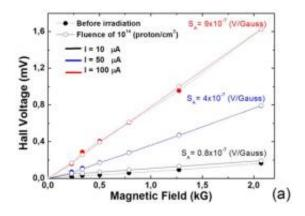
Variation of Hall voltage with magnetic field with drive current for an AlGaN/GaN Hall sensor before and after irradiation with proton fluence of 10 14 cm-2. Credit: Toyohashi University of Technology
