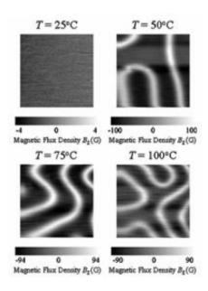
SHPM images of a bismuth substituted iron garnet thinfilms at 25-100 °C under an external perpendicular magnetic field Hext of 150 Oe. Credit: Toyohashi University of Technology
