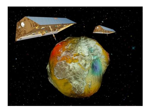
Twin-satellites GRACE with the earth's gravity field (vertically enhanceded) calculated from CHAMP data. © GFZ / Astrium
