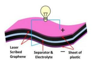
Schematic showing the structure of laser scribed graphene supercapacitors.
