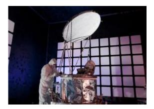
The Global Precipitation Measurement Microwave Imager (GMI) for NASA's Global Precipitation Measurement mission undergoes electromagnetic interference and compatibility testing at Ball Aerospace & Technologies Corp. Credit: Ball Aerospace
