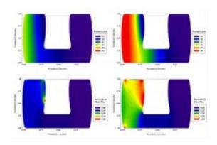
The University of Akron's Nicholas Garafolo accessed Ohio Supercomputer Center systems to characterize computational pressure profiles (top) and computational mass flux (bottom) of a potential main interface seal for docking at the International Space Station and other new spacecraft. Credit: Garafolo/UA
