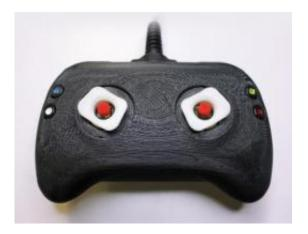
The University of Utah's latest prototype of a new kind of video game controller features typical thumb joysticks (white) but also has a round, red "tactor" in the center of each joystick to tug gently at the thumb tips. That kind of touch feedback is more advanced than existing games that vibrate the hands, and can simulate the tug of a fishing line, the feeling of ocean waves or the recoil of a gun. Credit: Markus Montandon, University of Utah
