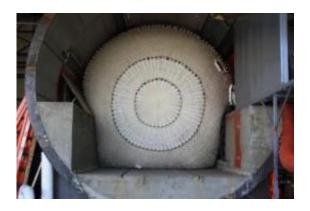
The plug uses high strength fabrics to withstand the pressures of a flooded tunnel. Credit: Photo by ILC Dover.
