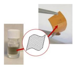
Single-layer graphene in solution used for making flexible transistors on a polyimide substrate (a sheet of thermostable polymer). Credit: CEA
