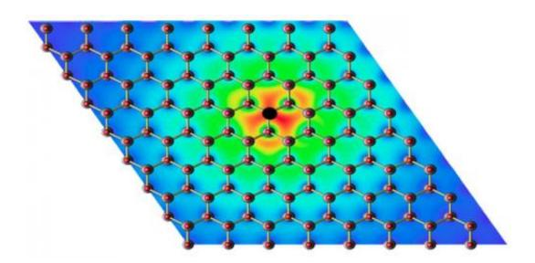
Visualization of the probability of finding an excited electron in zinc-oxide in the vicinity of the hole (indicated by the black dot). In order to understand the exciton in this transparent conducting oxide (TCO), the hole is assumed to be localized at an oxygen atom.
